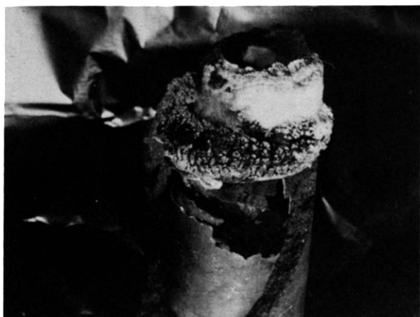
Fig. 3. 'Crystal' formed under nitrogen atmosphere.
